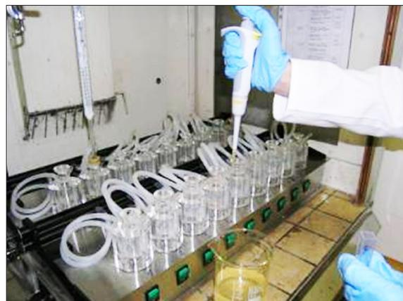
**Figure 1. B** - set of static diffusion cells.
