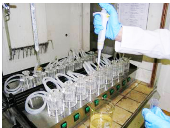
Figure 1. A - static diffusion cell: 1 – donor chamber, 2 – skin sample, 3 – sampling port, 4 – receptor chamber, 5 - manifold filling the water jacket, 6 – water (flow) jacket, 7 – magnetic stirrer.
