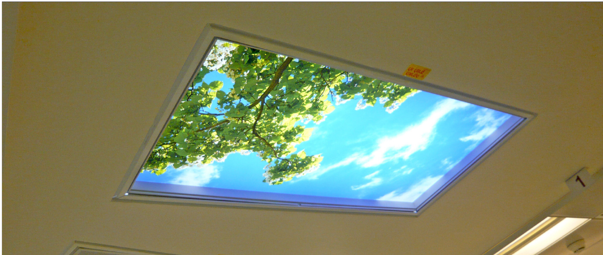
Figure 7. Artificial windows on ceilings reduce psychological stress for patients and personnel inhabiting underground spaces for long periods of time.
