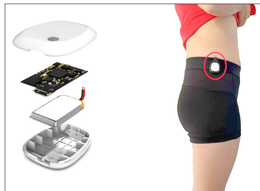
Figure 1. MBIENLAB MetaMotion device, actual size 27×27×4 mm (left), location on the body (right).
